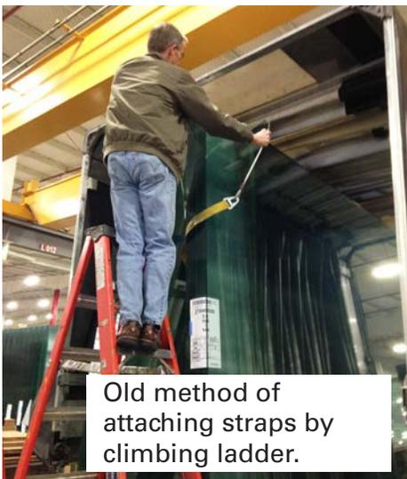
Old method of attaching straps by climbing ladder.
