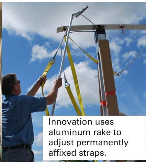
Innovation uses aluminum rake to adjust permanently affixed straps.
