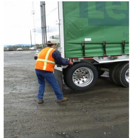
The driver should be watching for potholes in this wet gravel yard. Not cleaning off mud on his boot sole is a slip hazard for climbing into the cab.
