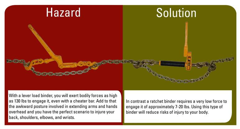
Lever load binders have been the tool for securing chains on loads for generations. Is there really a good reason to switch from a tool that has gotten the job done for years?
